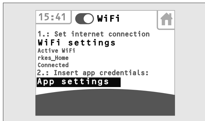
Fig. 3.34 Touch control panel – Wi-Fi receiver switched on
